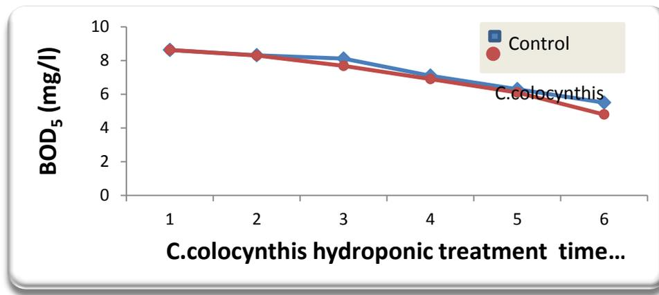
**Figure 5: Graphical representation of BOD<sub>5</sub> concentration treatment with treatment time**
