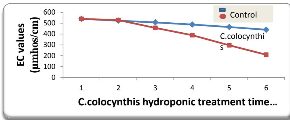
**Figure 3: Graphical representation of EC conc. Of treatment with treatment time**
