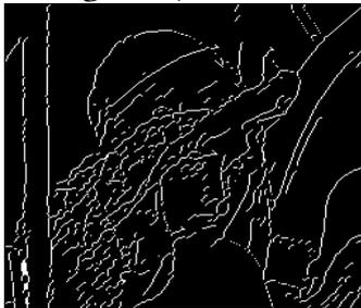
Figure 4: Output Result of the Suppressed Edges
