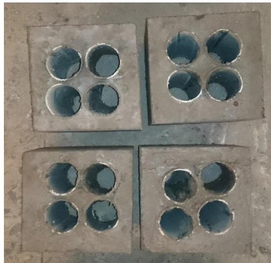
Plate 3.7: Square grid after de-molding operation
