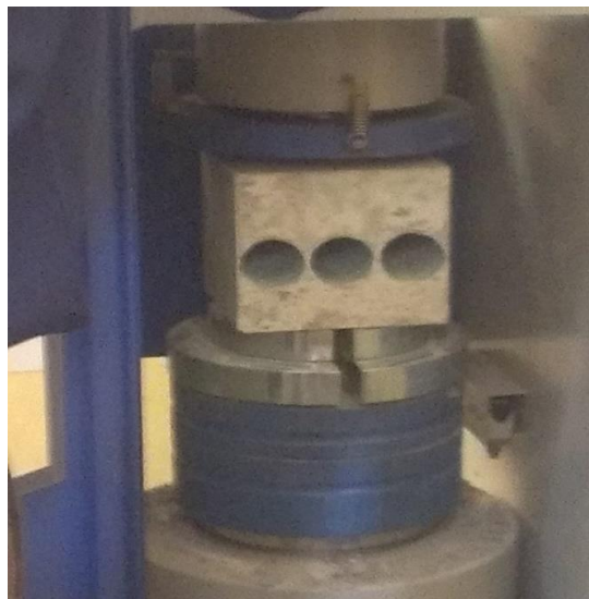
Plate 3.12: Compression machine in crushing operation Plate 3.13: Crushing of cube with PVC at edges
