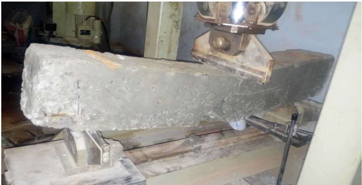
Plate 3.19: Beam failure under maximum applied load
