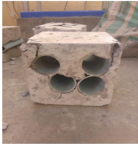
Plate 3.9: Failure pattern at edges
