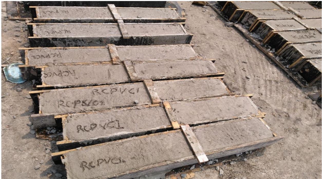
Plate 3.16: Casting of Concrete with and without PVC pipes
