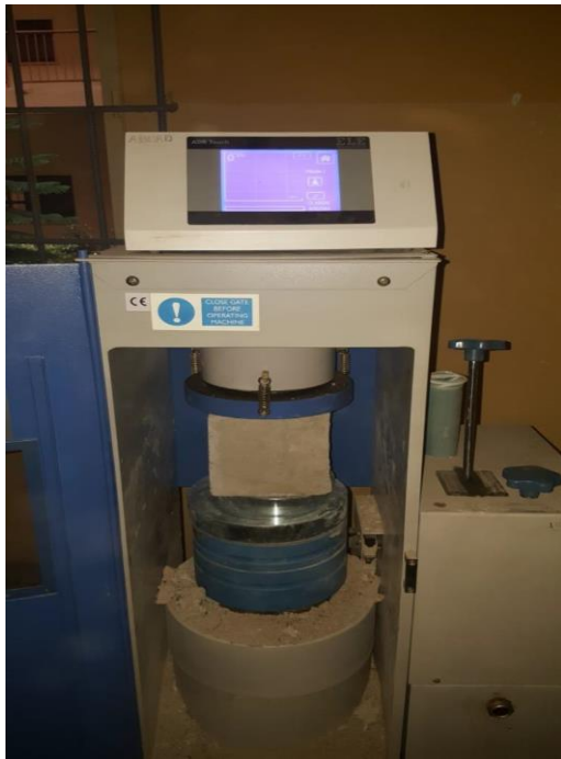
Plate 3.12: Compression machine in crushing operation Plate 3.13: Crushing of cube with PVC at edges
