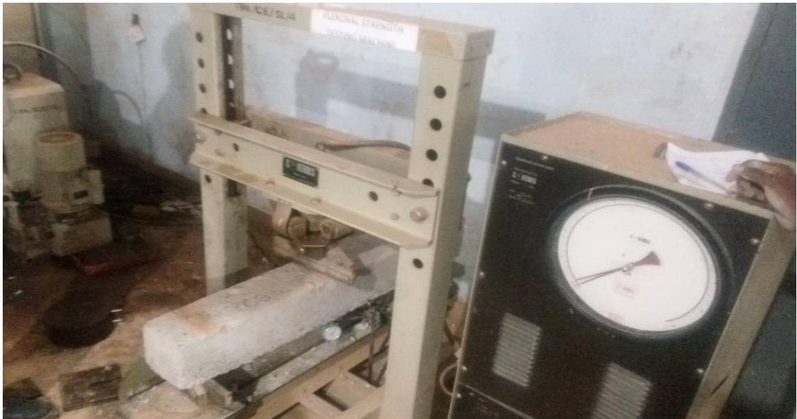
Plate 3.18: Experimental set up (ASTM 293 C) with force units attached
