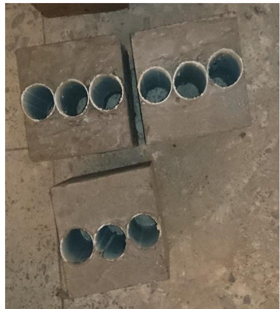
Plate 3.11: De-molding of centre grid pattern
