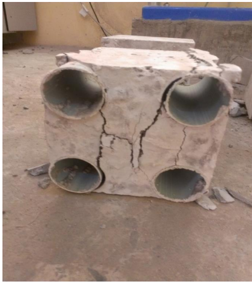
Plate 3.8: Failure pattern for square grid at edges
