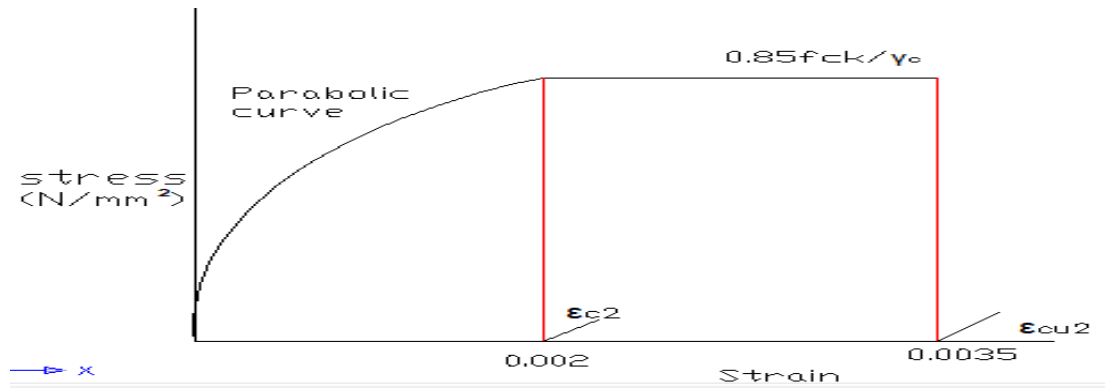
Figure 2.3: Parabolic-rectangular stress-strain diagram for concrete in compression
