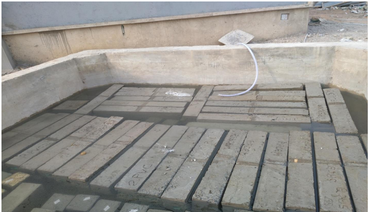
Plate 3.17: Beams in curing Tank
