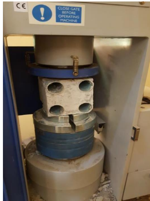
Plate 3.12: Compression machine in crushing operation Plate 3.13: Crushing of cube with PVC at edges
