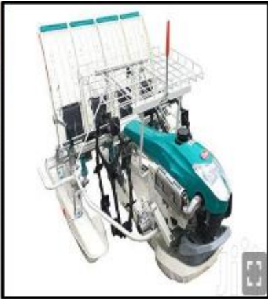
Figure 3B: Motorised Four Rows Rice Seedling Transplanter ( www.jiji.ng ).
