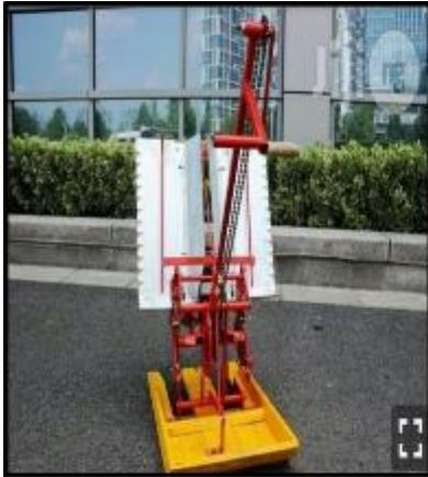
Figure 3A: Manually Operated Two Rows Rice Seedling Transplanter ( www.jiji.ng ).
