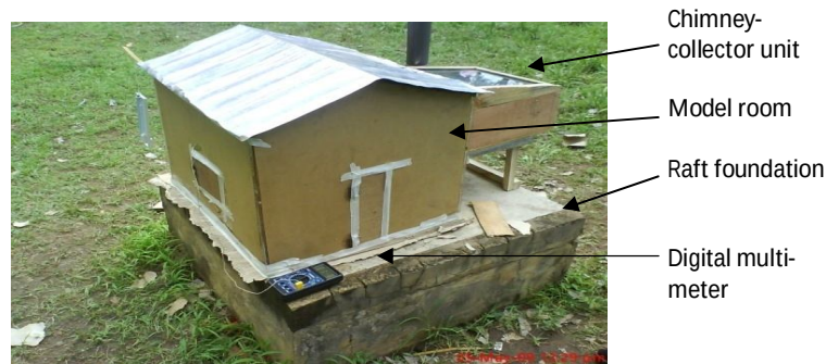
Figure 5 Model building with the attached solar chimney-collector
