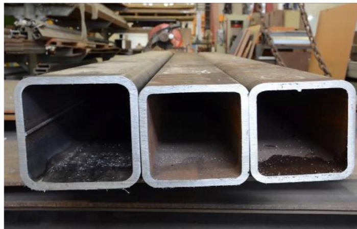
Figure 3.17b: Steel Hollow Section for Cold-Formed Column EN10219 1997
