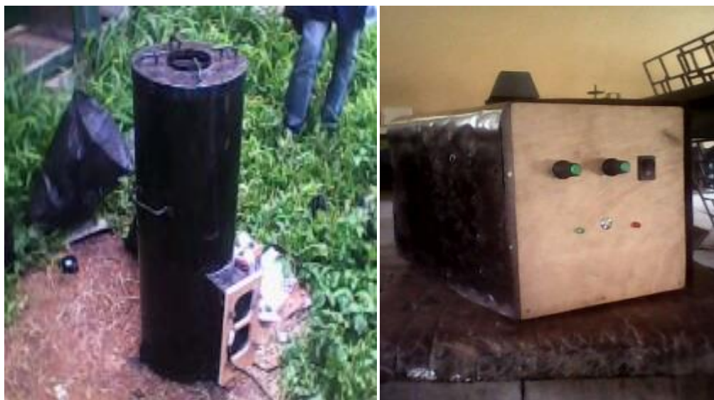
Fig. 4. Completed Stove and Power Supply Unit
