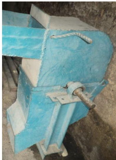
Fig.1b. A locally fabricated commercial hammer mill in Bodija Market, Ibadan
