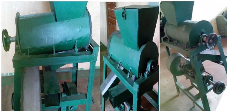
Figure 4. The combined maize dehulling, cleaning and milling machine
