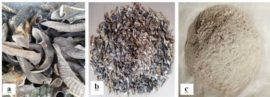
Plate 1: (a) Ovisaries horn (b) Ovisaries horn chips (c) Ovisaries horn particles
