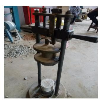
Figure 5: Aggregate impact testing machine.
