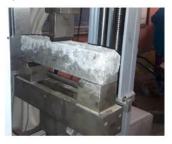
Figure 3: Determination of flexural strength of the concrete.
