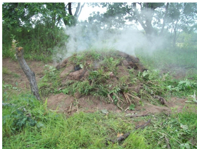
Figure 3.3: The process of destructive distillation wood to produce charcoal.
