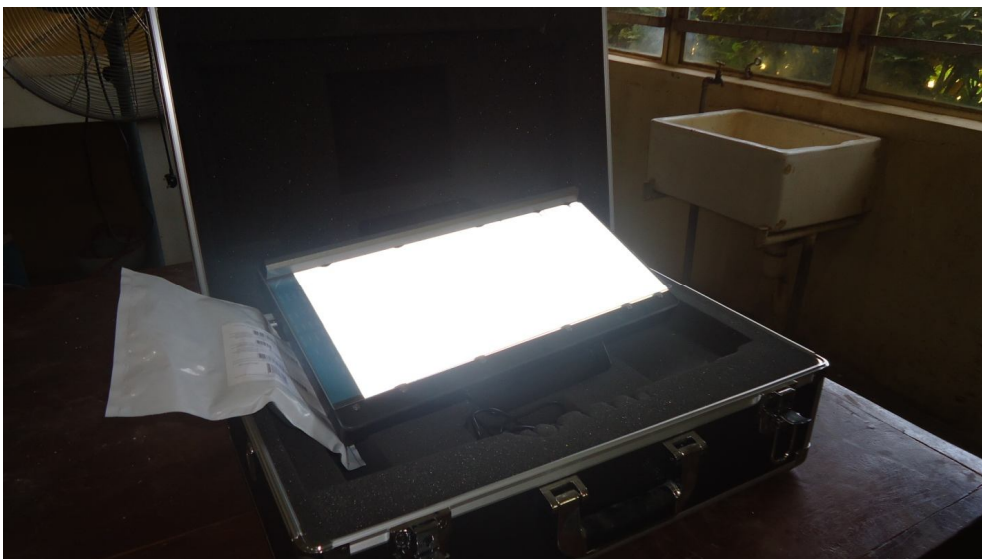
Portable Leaf Area Meter: An instrument for determining surface area of leaves.
