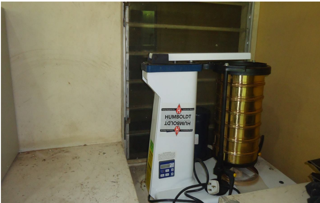
Motorized Sieve Shakers: An instrument for determining the particle size of materials/products
