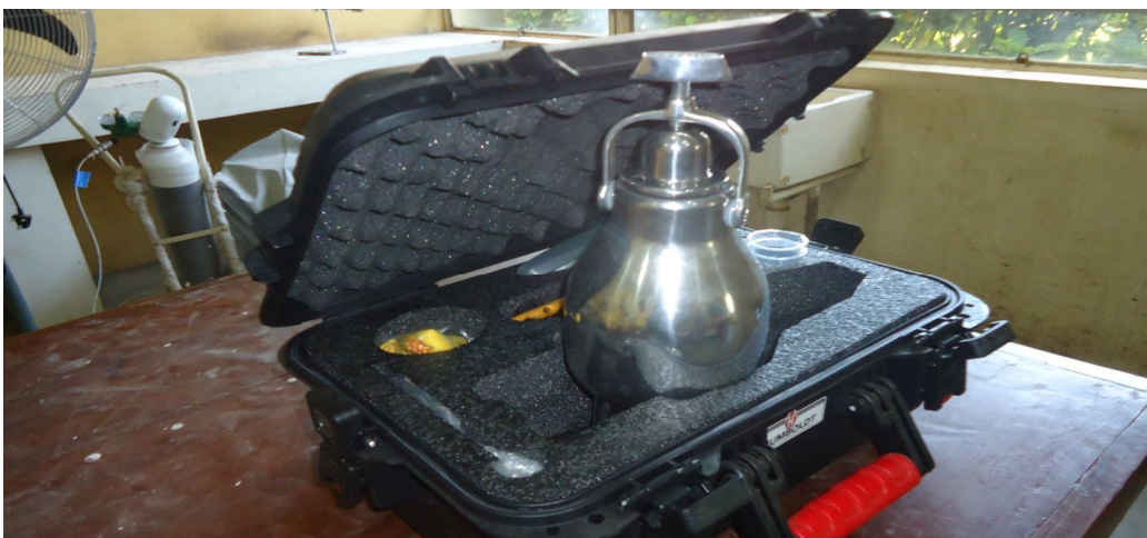
Moisture Meter: An instrument for determining the moisture content of materials
