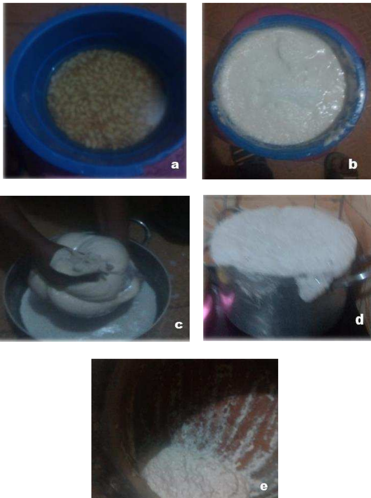
Figure 1: Soaked Soyabeans (a) Grinded Soya (b), Sieving of Soya beans (c), Cooking of Soya beans (d) and (e) soy adhesive
