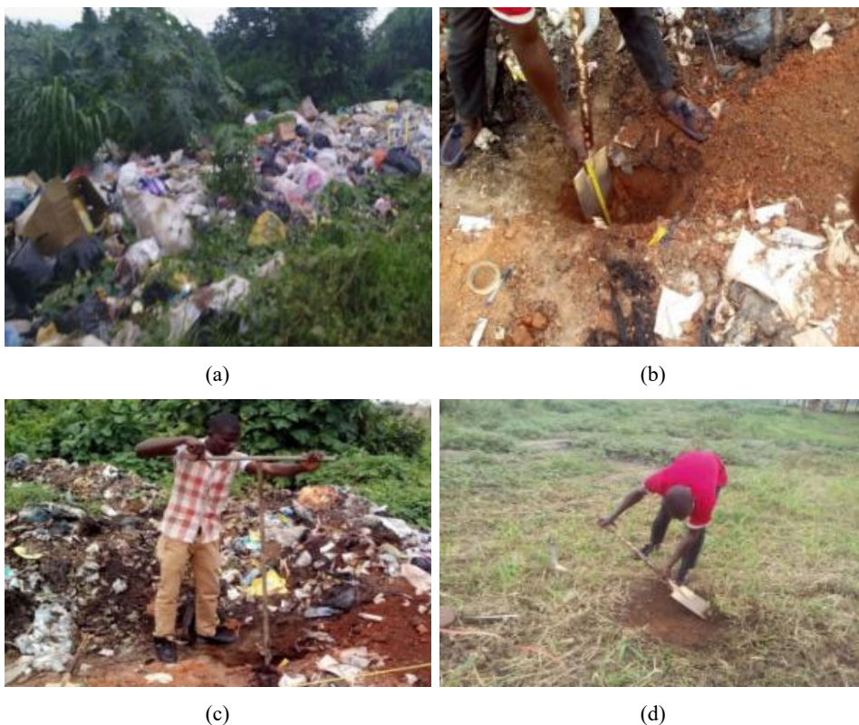
Figure 2 Soils sampling, (a) Igbaturo dumpsite (b) depth measurement to obtain samples (c) use of soil auger to obtain samples at different depths on a spot (d) use of shovel to remove grasses to obtain control samples (20 m away from dumpsite) (see online version for colours)
