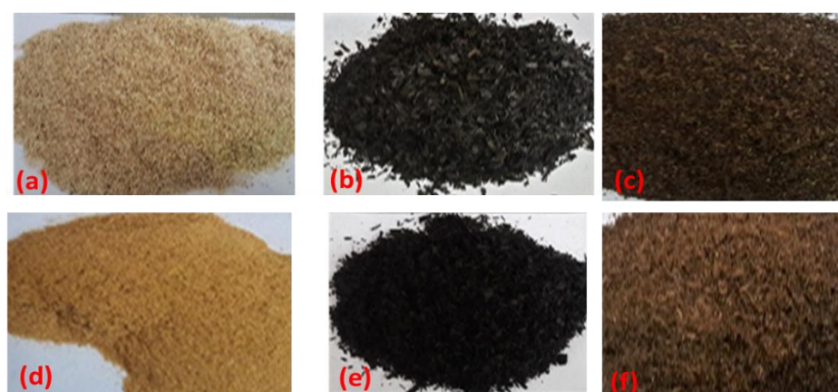
Figure 4.11: Colours of; (a) raw Melina wood (b) severely torrefied Melina wood (c) mildly torrefied Melina wood (d) raw Teak wood (e) severely torrefied Teak wood and (f) mildly torrefied Teak wood.
