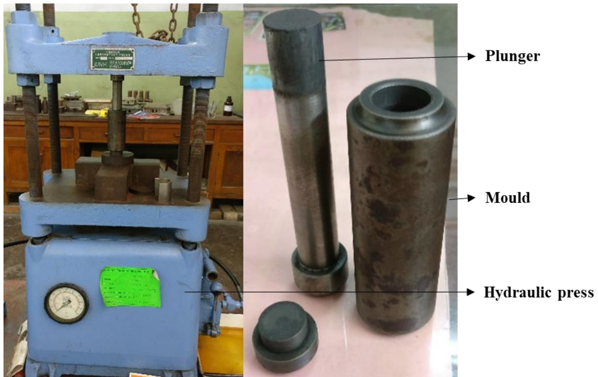
Figure 3.4: Briquetting machine and its components
