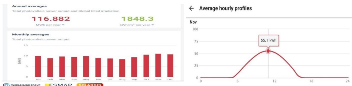
Fig. 3. The monthly and hourly distribution of the photovoltaic power output in PV Grid Region A
