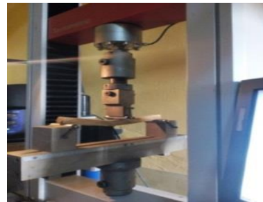
Figure 2: Bending Test arrangement
