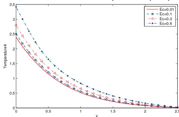
Figure 3. The thermal distribution profiles with variation of Eckert number  $Ec$  at time  $t=0.6$  and for fixed parameters  $Pr=0.71$ ,  $F=1$ ,  $G=8$  and  $M=1$
