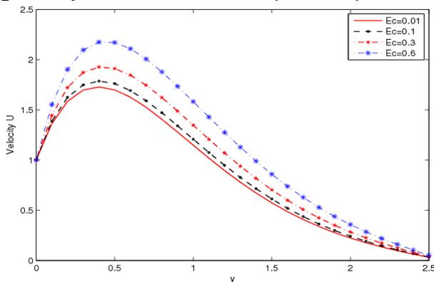
Figure 1. The velocity distribution profiles with variation of Eckert number  $Ec$  at time  $t=0.6$  and for fixed parameters  $Pr=0.71$ ,  $F=1$ ,  $G=8$  and  $M=1$
