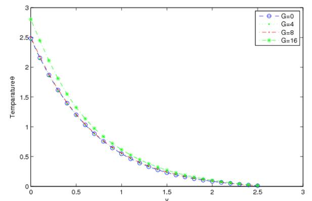
Figure 4. The thermal distribution profiles with variation of Grashof number  $G$  at time  $t=0.4$  and for fixed parameters  $Pr=0.71$ ,  $F=1$ ,  $Ec=0.1$  and  $M=1$
