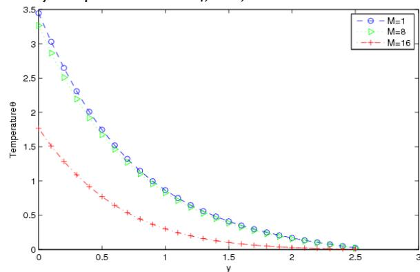
Figure 9. The thermal distribution profiles with variation of magnetic field parameter  $M$  at time  $t=0.8$  and for fixed parameters  $Pr=0.71$ ,  $F=1$ ,  $Ec=0.1$  and  $G=8$
