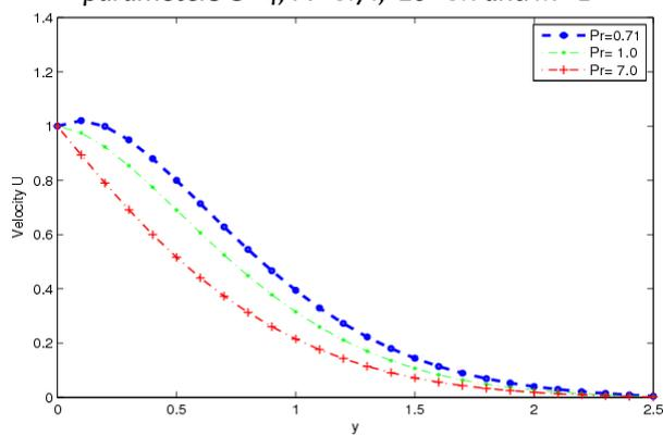
Figure 7. The velocity distribution profiles with variation of Prandtl number  $Pr$  at time  $t=0.4$  and for fixed parameters  $G=4$ ,  $F=1$ ,  $Ec=0.01$  and  $M=1$
