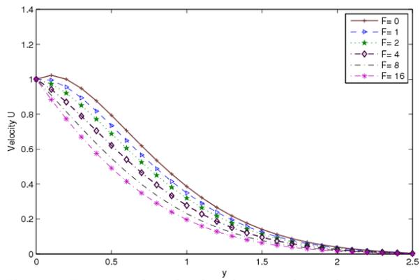
Figure 5. The velocity distribution profiles with variation of radiation parameter  $F$  at time  $t=0.4$  and for fixed parameters  $G=4$ ,  $Pr=0.71$ ,  $Ec=0.1$  and  $M=2$
