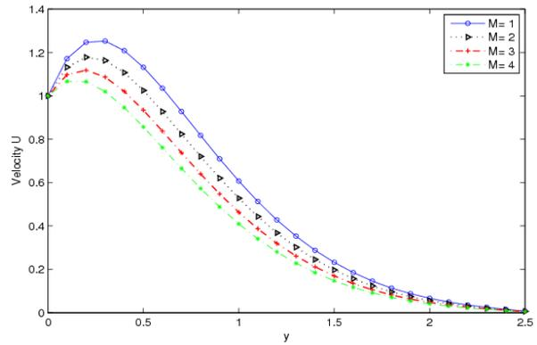
Figure 6. The velocity distribution profiles with variation of magnetic field parameter  $M$  at time  $t=0.4$  and for fixed parameters  $Pr=0.71$ ,  $F=1$ ,  $Ec=0.1$  and  $G=8$
