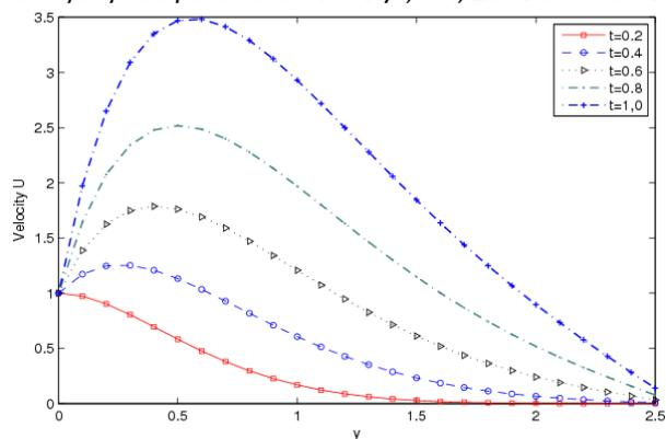
Figure 11. The velocity distribution profiles with variation of time for fixed parameters  $Pr=0.71$ ,  $F=1$ ,  $Ec=0.1$  and  $G=8$
