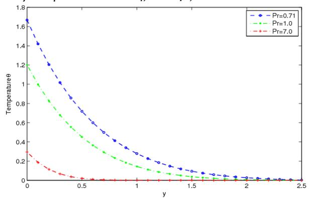
Figure 10. The thermal distribution profiles with variation of Prandtl number  $Pr$  at time  $t=0.4$  and for fixed parameters  $G=4$ ,  $F=1$ ,  $Ec=0.01$  and  $M=1$
