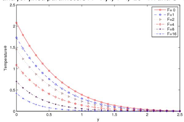
Figure 8. The thermal distribution profiles with variation of radiation parameter  $F$  at time  $t=0.4$  and for fixed parameters  $G=4$ ,  $Pr=0.71$ ,  $Ec=0.1$  and  $M=2$
