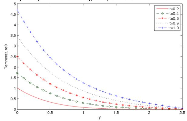
Figure 12. The thermal distribution profiles with variation of time for fixed parameters  $Pr=0.71$ ,  $F=1$ ,  $Ec=0.1$  and  $G=8$
