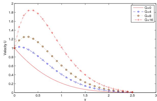
Figure 2. The velocity distribution profiles with variation of Grashof number  $G$  at time  $t=0.4$  and for fixed parameters  $Pr=0.71$ ,  $F=1$ ,  $Ec=0.1$  and  $M=1$ .
