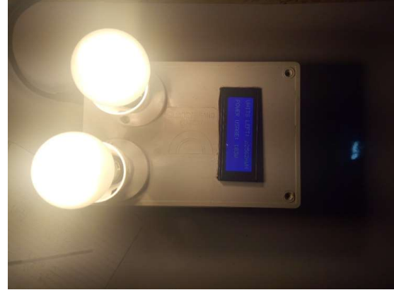
Plate 2: Meter Reading with Two 60 W Rated Load
