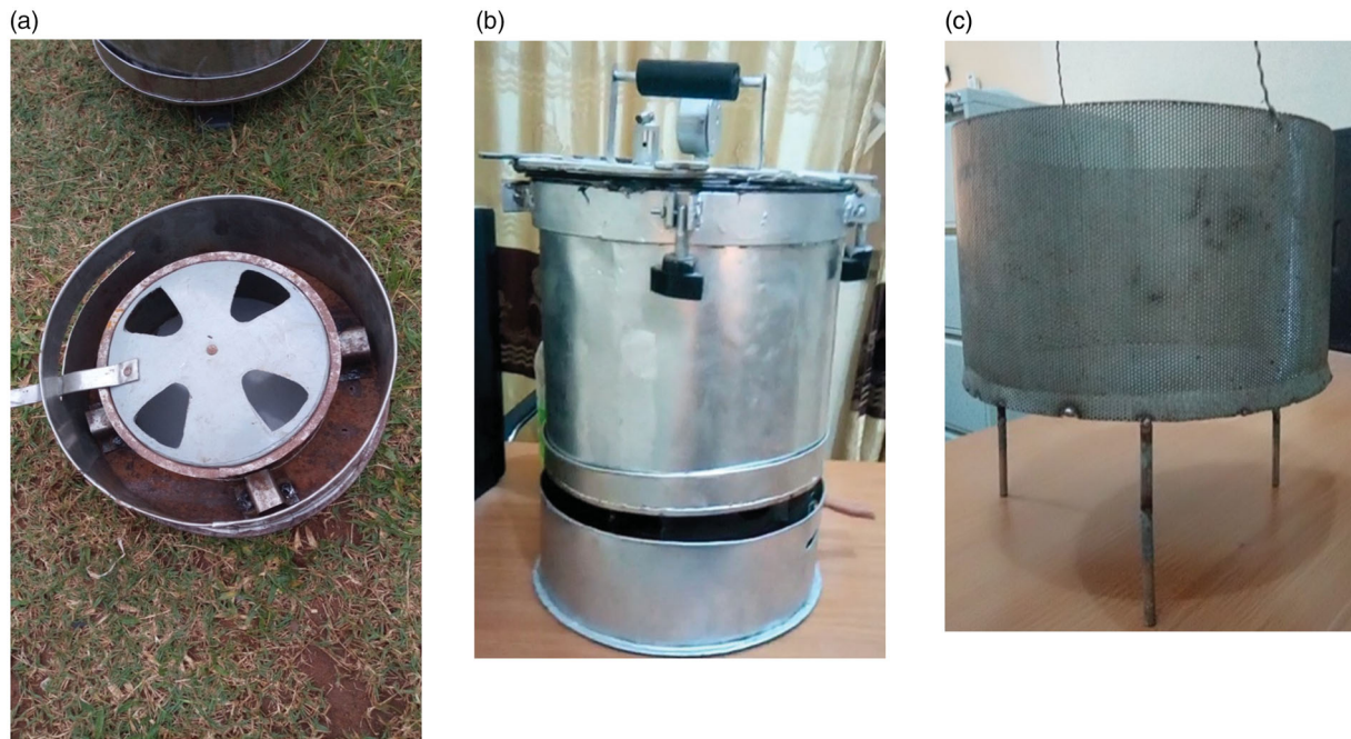
Figure 2. Images of the main parts of the designed autoclave. (a) Cook stove; (b) Autoclave; (c) Canister.
