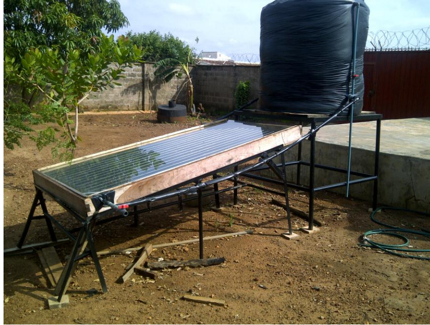
FIGURE 4: PICTURE OF THE SOLAR WATER HEATER
