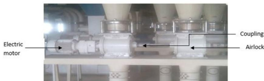
**Figure 1.** The coupling during operation
