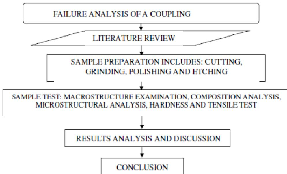
**Figure 3.** Flow diagram of the study
