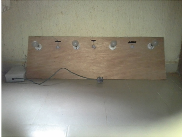
Figure 8: Assembled project showing luminaires and sensors.
