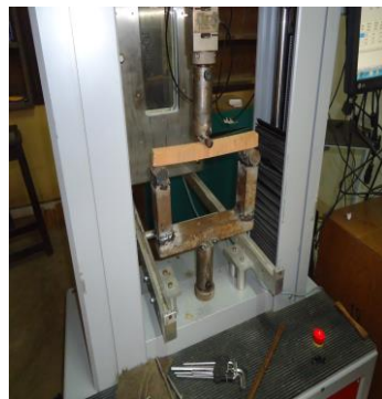
Figure 4: (a) Bending test set up (b) Failure mode
