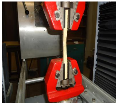
(a) Tensile test set up
