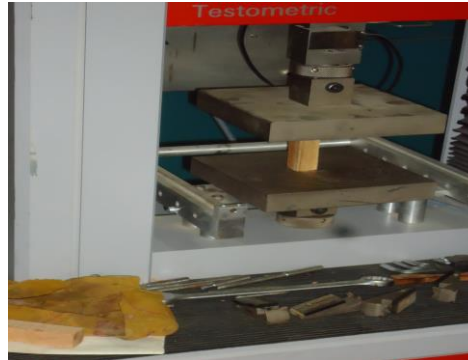
Figure 3: Compression test set up
