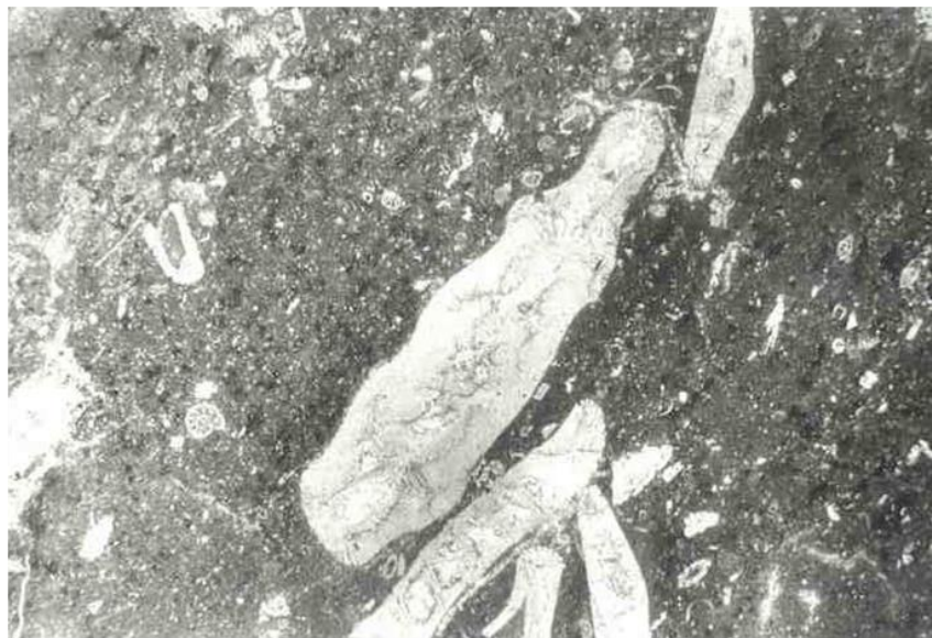
Figure 4. Photomicrograph of bioclastic wackestone. Notice the big grain of larger foraminifera (LF) at the center of photo. Notice also the transverse section of echinoderm (E) at the top left of photo.
