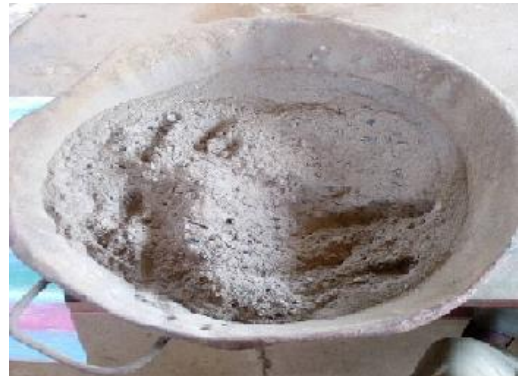
Fig. 2.2: Controlled furnace used for PKS incineration Fig.2.3 Processed PKS ash
