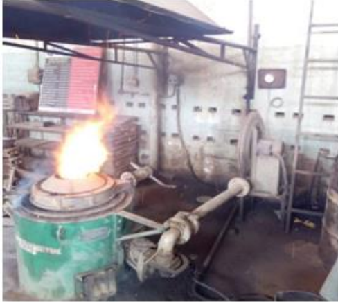
Fig. 2.2: Controlled furnace used for PKS incineration Fig.2.3 Processed PKS ash
