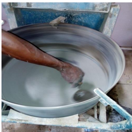
Fig. 2.4: The process of inter-grinding by electric machine
