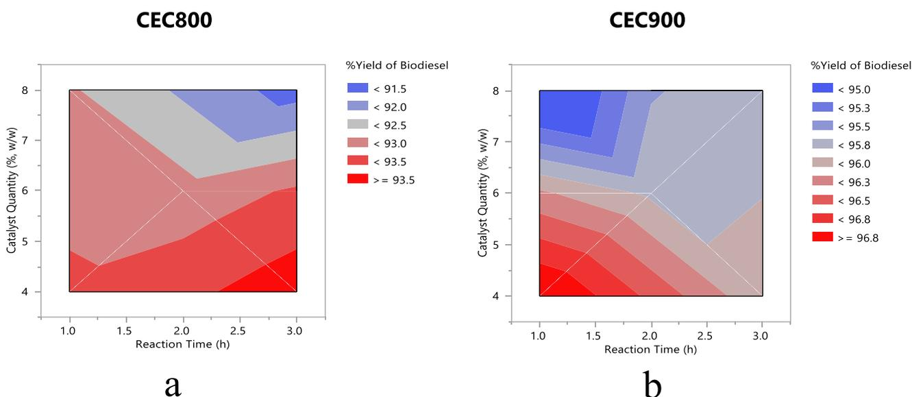
**Fig. 9** %Yield of PBD by interaction between catalyst quantity and reaction time for CEC800 and CEC900
