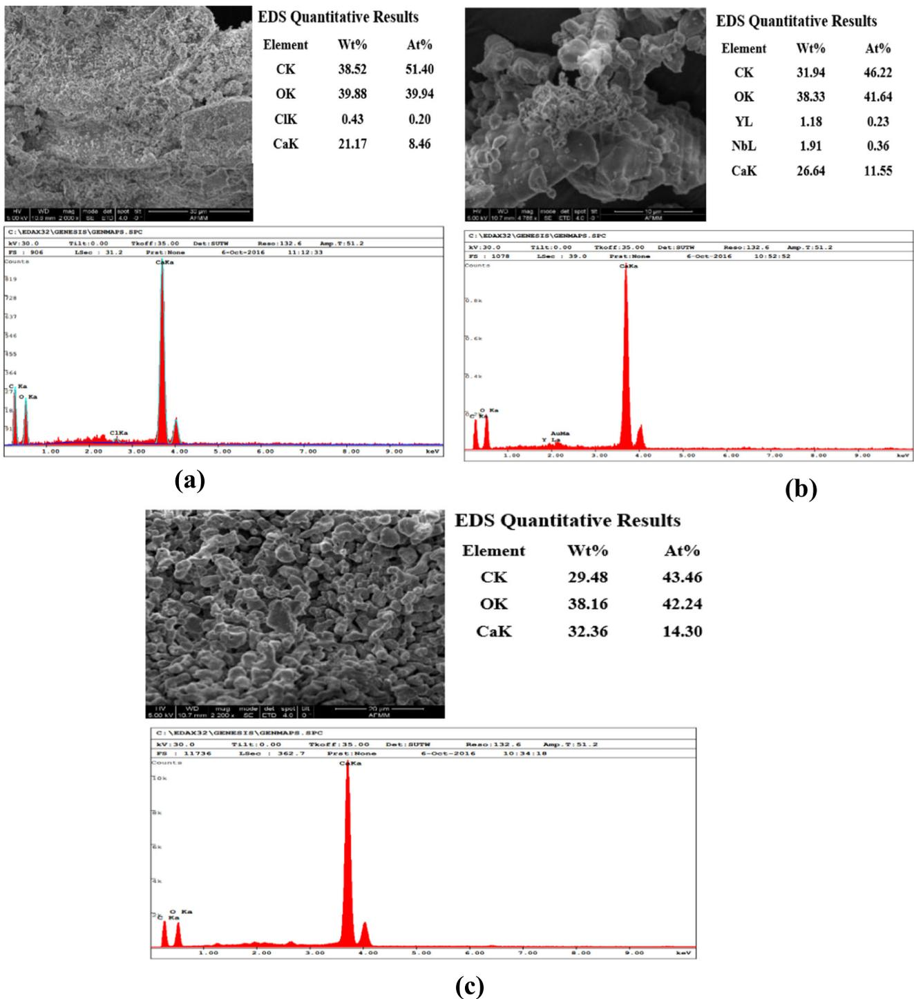
Fig. 4 The morphology structure and EDS of **a** chicken eggshell (Ajala, Eletta, et al., 2018), **b** CEC800, and **c** CEC900
