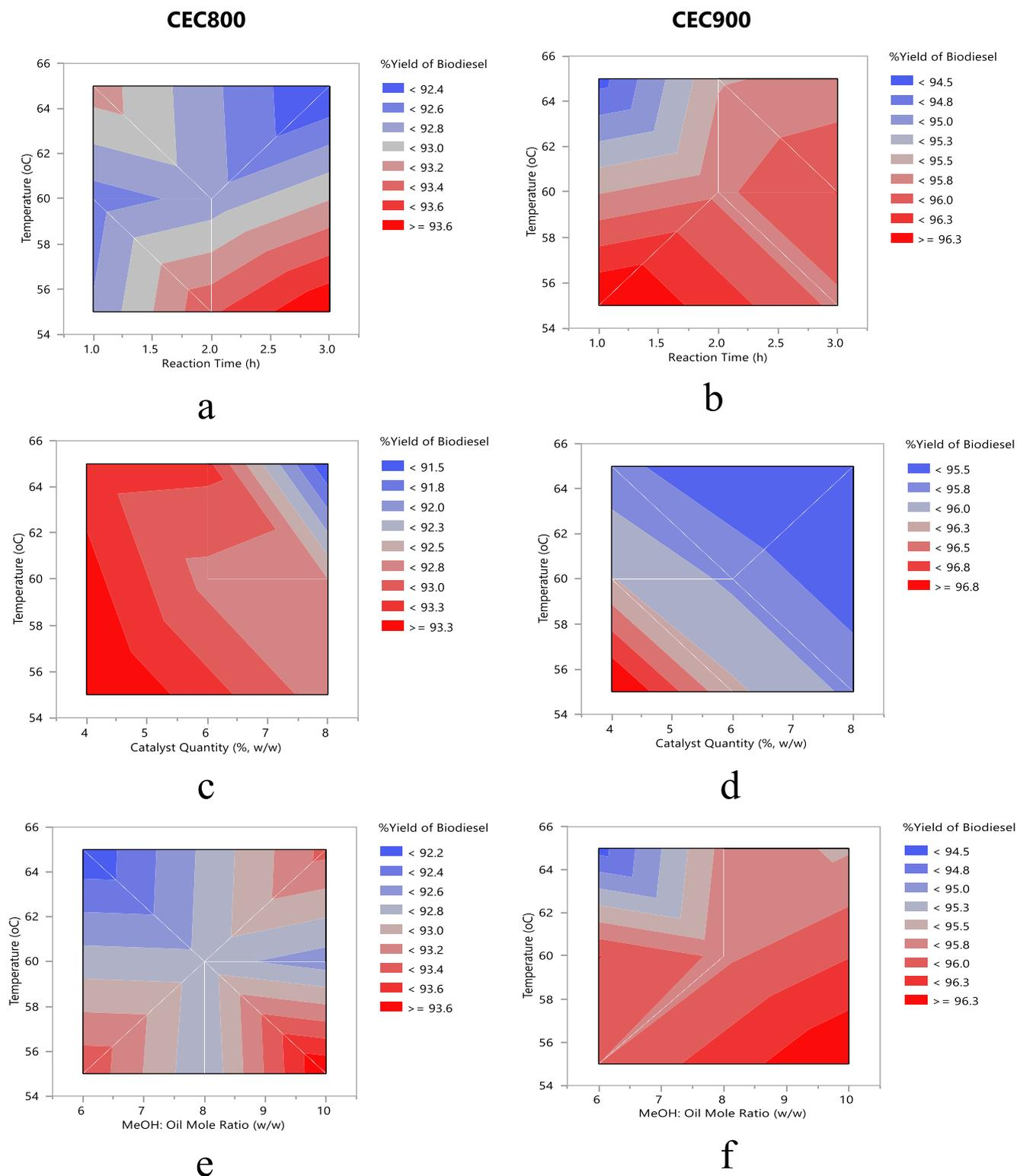
**Fig. 8** %Yield of PBD by interaction between temperature ( $^{\circ}\text{C}$ ) and other parameters for CEC800 and CEC900
