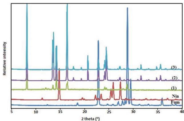
**Figure 2.** XRPD pattern of fumaric acid, nicotinamide,  $[\text{Cu}(\text{H}_2\text{O})_4(\text{Nia})_2](\text{Fum}) \cdot (\text{H}_2\text{Fum})$  (1),  $[\text{Co}(\text{H}_2\text{O})_4(\text{Nia})_2](\text{Fum}) \cdot (\text{H}_2\text{Fum})$  (2), and  $[\text{Ni}(\text{H}_2\text{O})_4(\text{Nia})_2](\text{Fum}) \cdot (\text{H}_2\text{Fum})$  (3).
