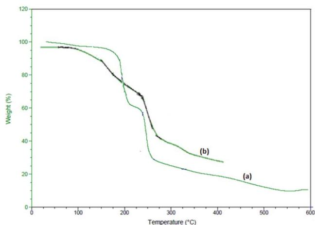
**Figure 1.** The TGA curve for (a) [Cu(H<sub>2</sub>O)<sub>4</sub>(Nia)<sub>2</sub>](Fum)·(H<sub>2</sub>Fum) (**1**) and (b) [Ni(H<sub>2</sub>O)<sub>4</sub>(Nia)<sub>2</sub>](Fum)·(H<sub>2</sub>Fum) (**3**).
