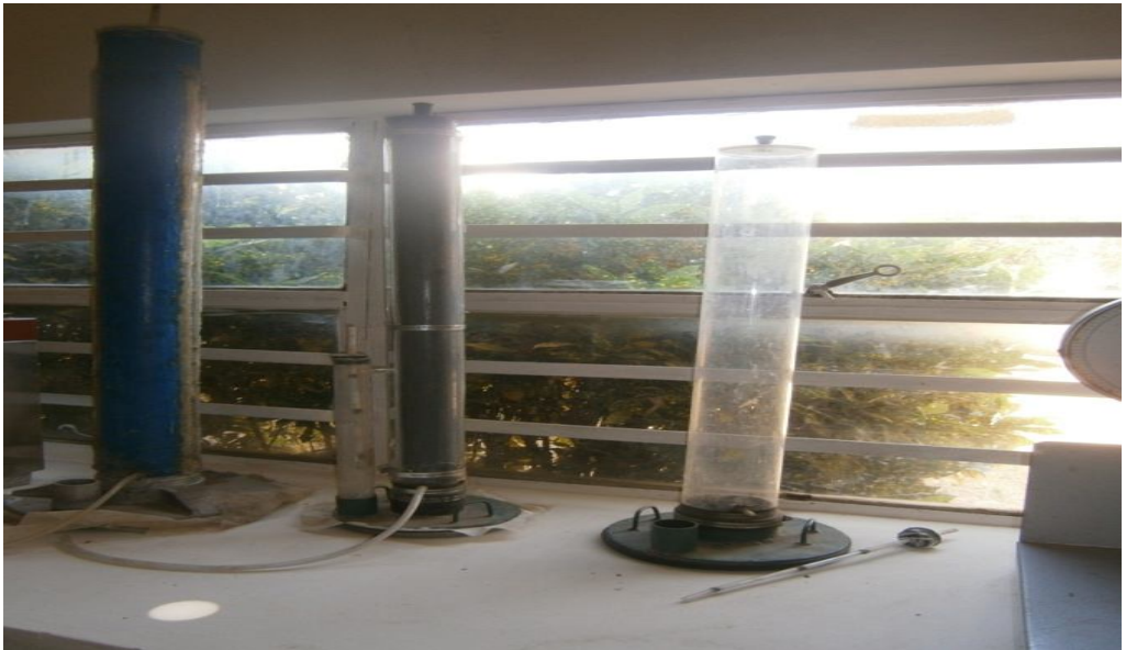
INFILTROMETERS. A device used to measure the rate of water infiltration into soil or other porous media.
