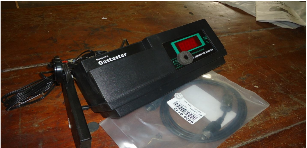
GUNSON DIGITAL EXHAUST GAS ANALYZER ( Model- G4125). An instrument for the testing and setting of all carburettors (petrol, leaded or unleaded) and petrol injection systems on any vehicle
