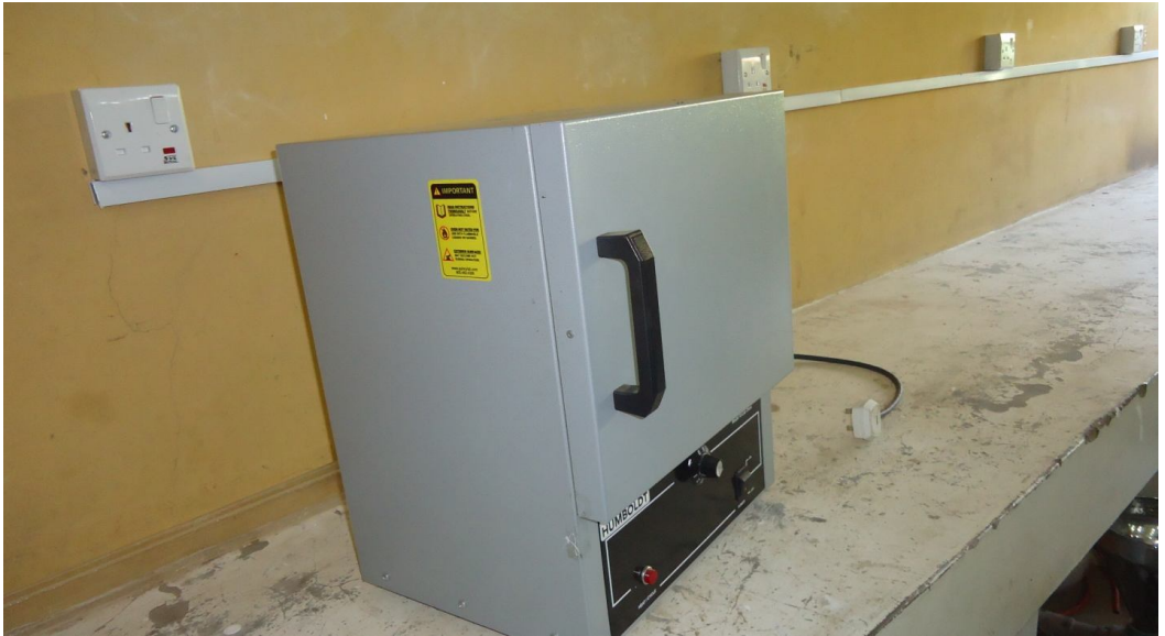
Laboratory Oven Model H-30100.4F (O°-300°): An instrument for determining the moisture content of agricultural and biological materials.
