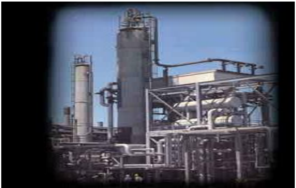
Gas absorption column: hydrogenation of oils
