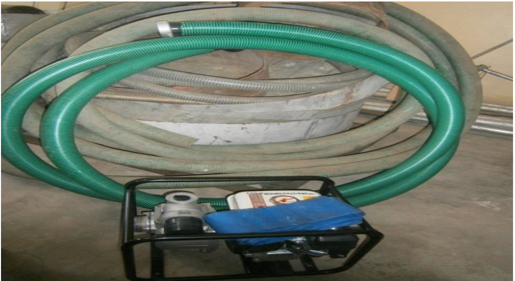
WATER PUMP AND SUCTION HOSES. Instruments that lift and conduct the water from the source (lake, river, pond, etc.) to the pump.
