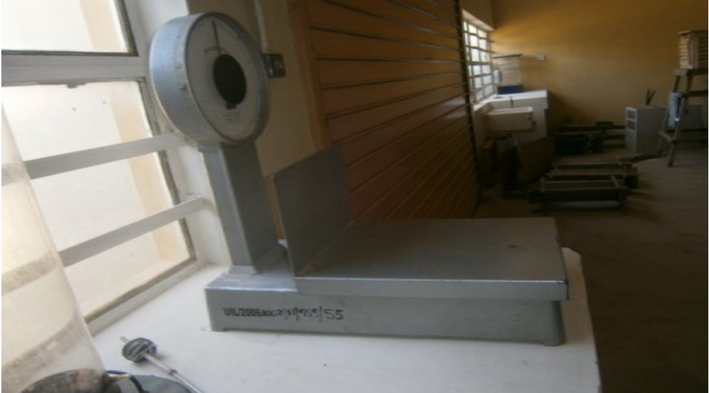
Weighing Scale: An instrument that measures the weight of an item
