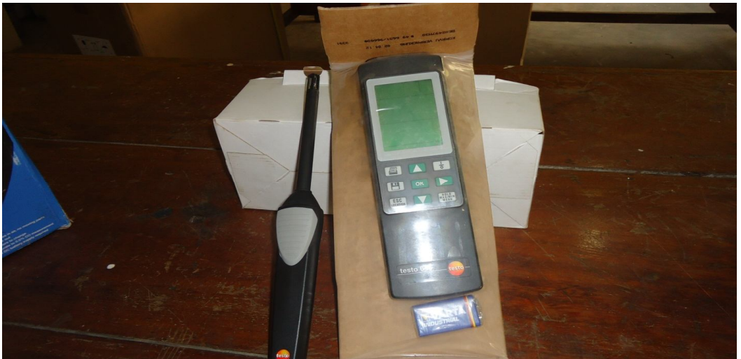
TESTO 645 Temperature and Relative Humidity Measurement Data Logger with probe_ A device for measuring temperature and relative humidity of produce in a structure.
