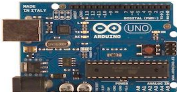
Arduino Board: A module which basically allow for control of appliances
