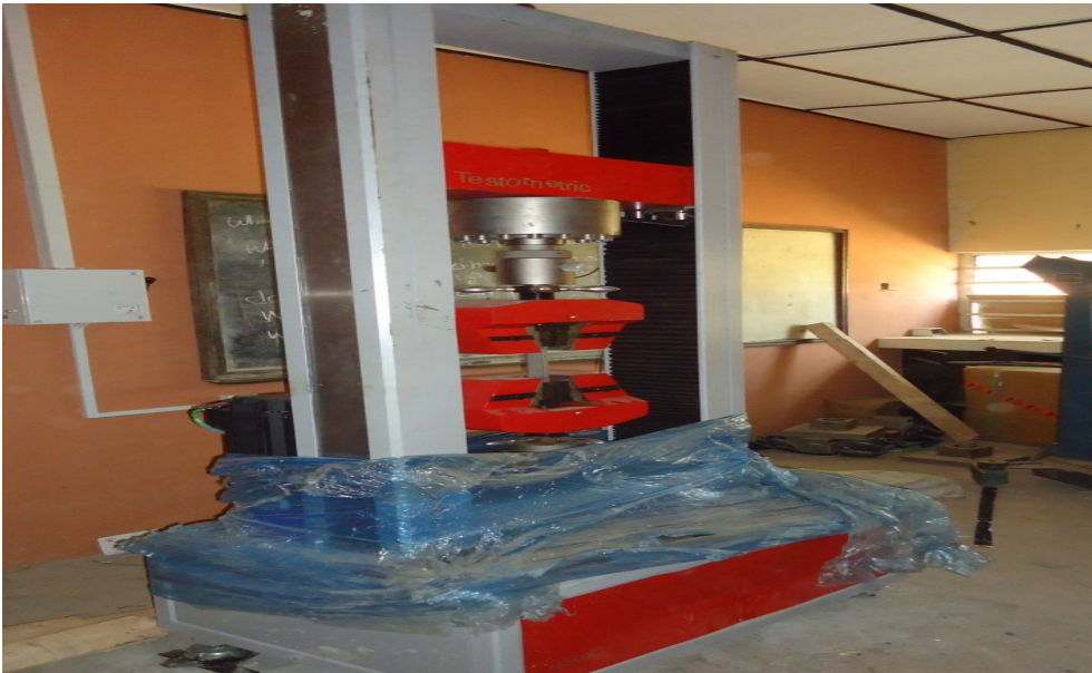
Testometric Universal Testing Machine (TUTM) : A tool for determining the mechanical properties of agricultural and biomaterials
