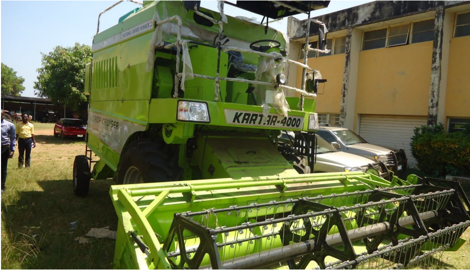
Kartar 4000 (41") Multicrop Combine Harvester A machine that harvest grain crops.
