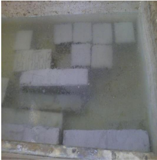
Figure 1: Curing process of cube specimen
