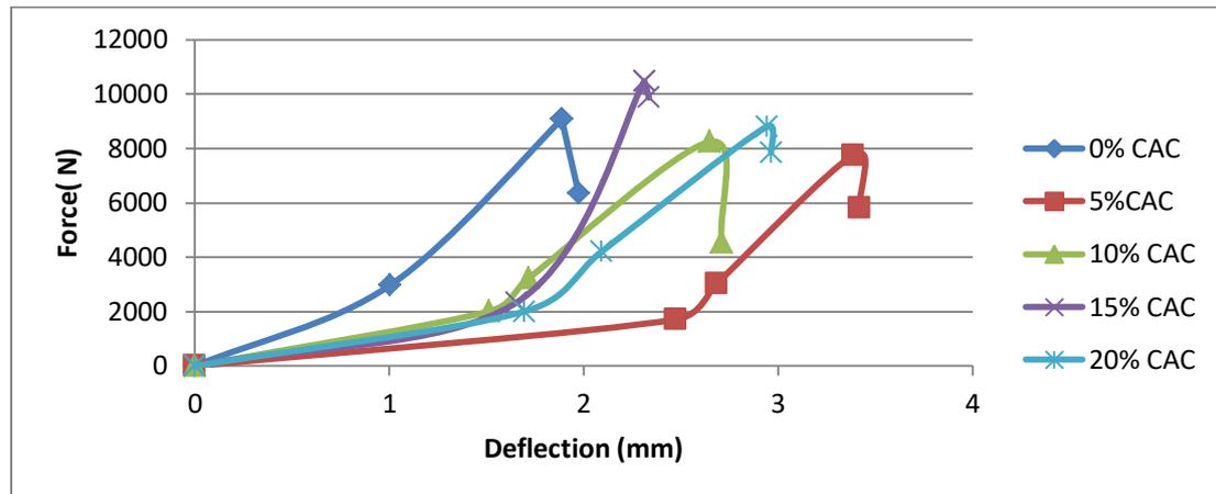
Figure 11: Flexural load deflection curve for calcium carbide waste (CCW) in concrete beams
