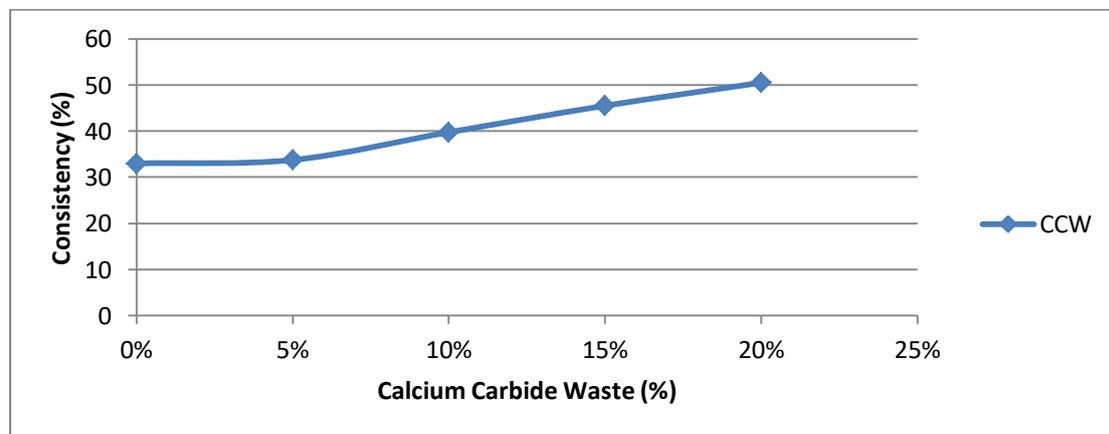
Figure 7: Consistency of the Mix with Cement Replacement
