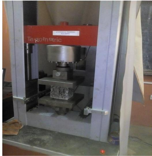
Figure 2: Process of testing cube specimen
