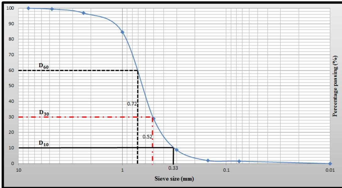
Figure 5: Particle size distribution curve of fine aggregate.
