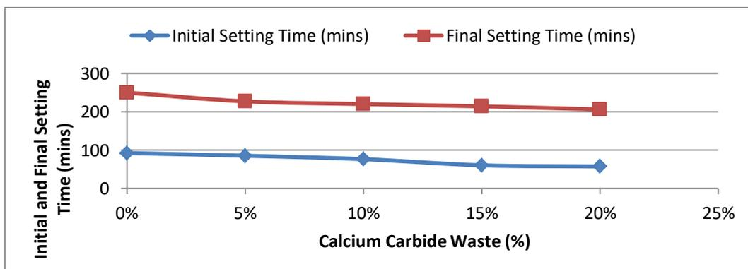
Figure 6: Initial and Final Setting Time of Calcium carbide waste (CCW) Mortar
