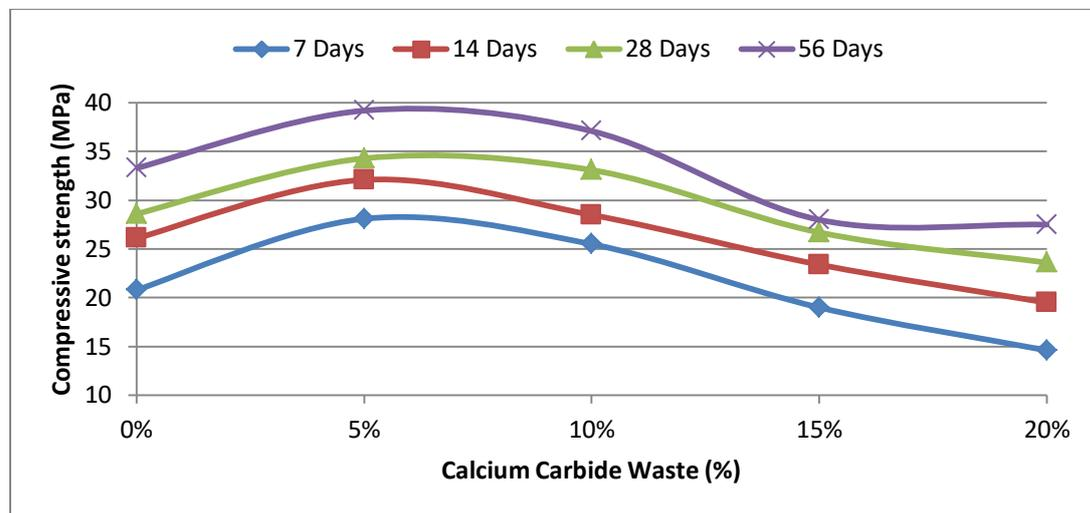
Figure 8: Rate of Strength Development with Cement Replacement
