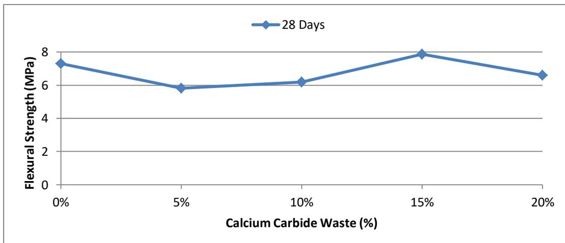
Figure 10: Rate of Change in Flexural Strength with Cement Replacement
