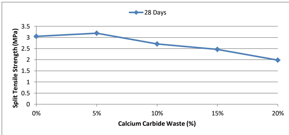
Figure 9: Rate of Change in Tensile Strength with Cement Replacement
