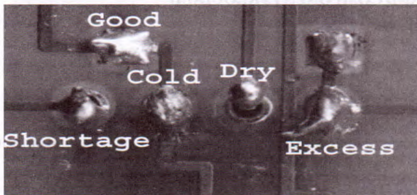
Figure 1.1: Examples of Joints
